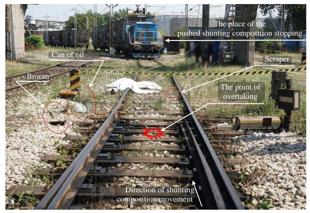
**Figure 3.2.1:** The appearance of the place of the serious accident after the overtaking of the pushed shunting composition on the railway worker (view from the direction of the second track to the second turnout track)
