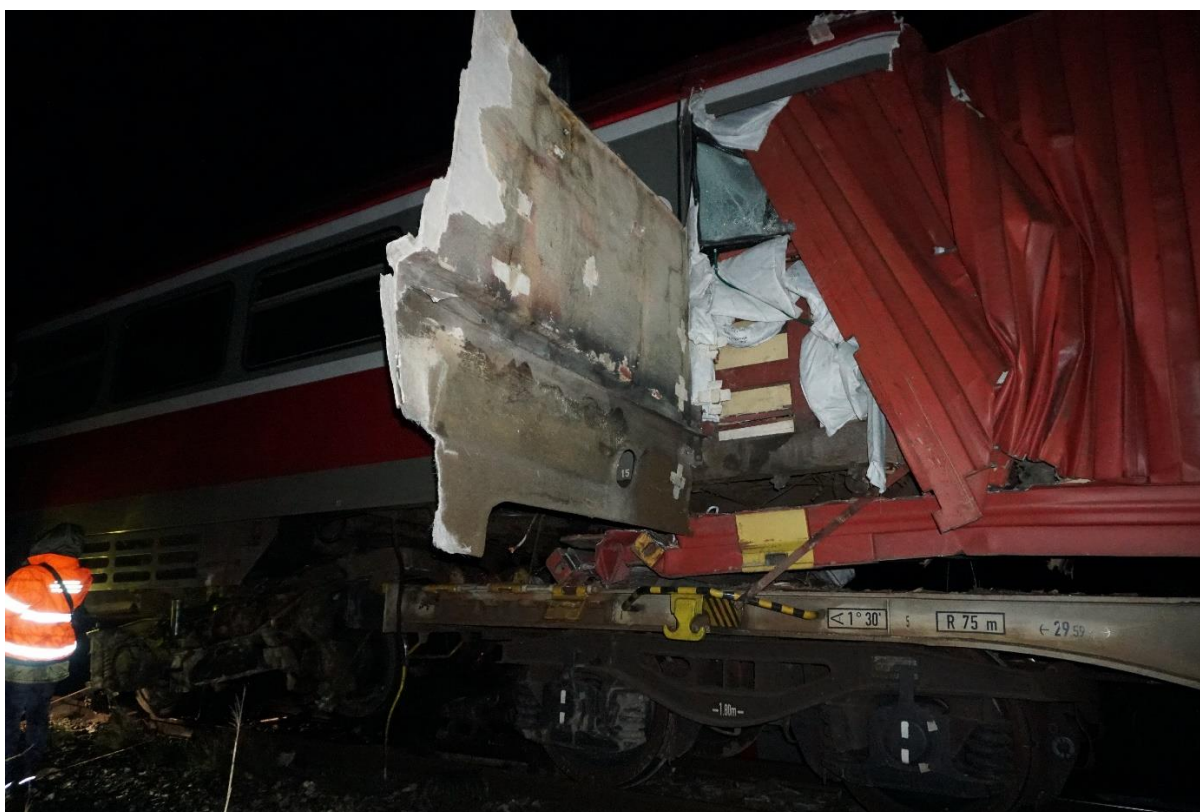
Figure 4.1.1.2: The appearance of the damages on the front box part of DMV 711-078 and on the container CNEU 453486-3
