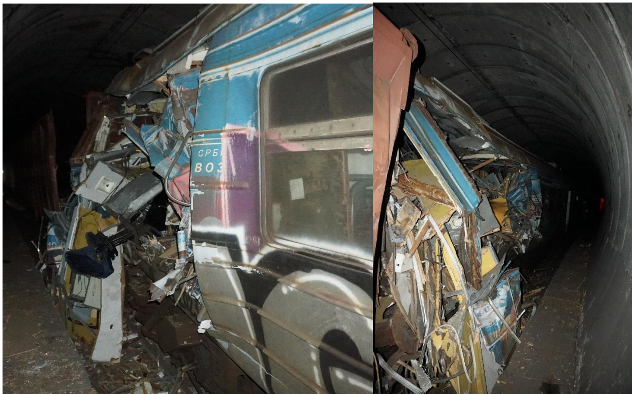
Figure 3.1.1: Appearance of the damage on the front part of the motor coach 412-005 of the train No. 7112 after the accident
