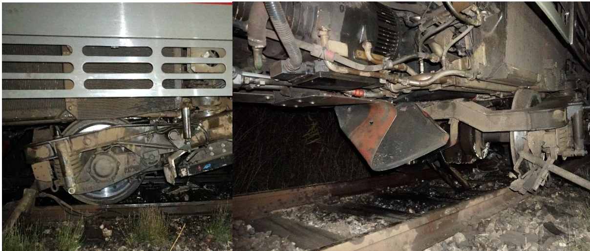
Figure 4.1.1.5: Appearance of damages on the power unit DMV 711-078
