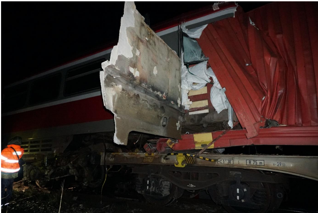
Figure 3.1.2: The appearance of the damages on the front DMV box part 711-078 and on the container CNEU 453486-3
