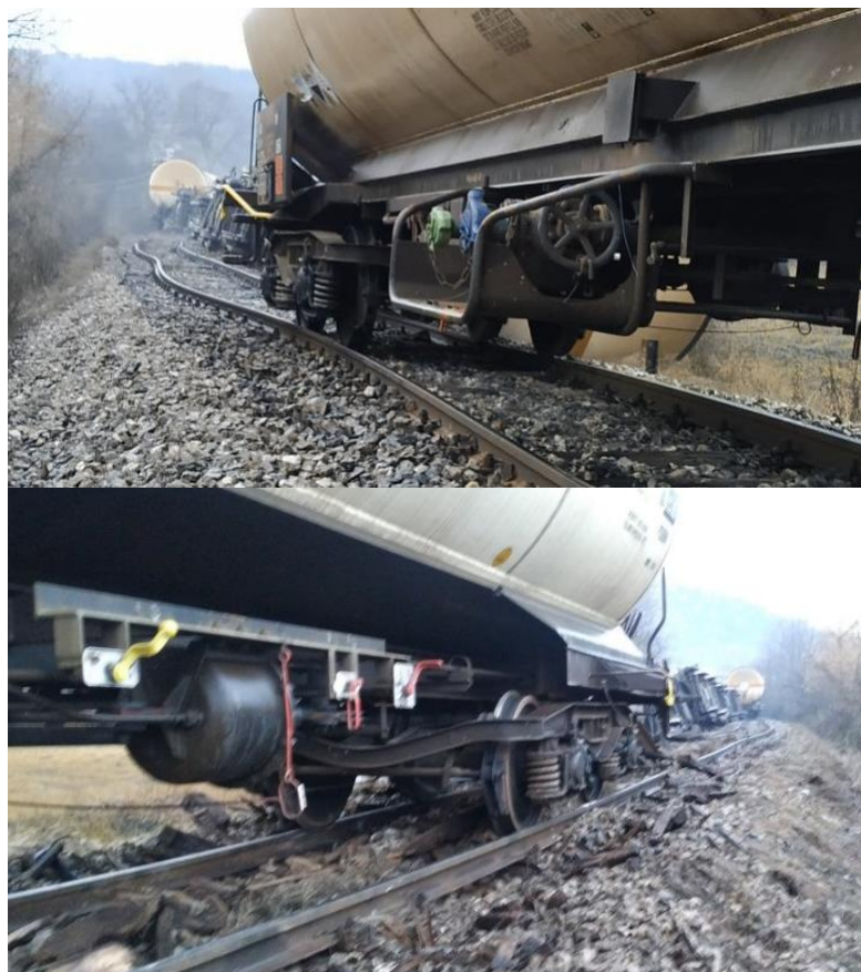
Figure 4.1.1.4: The appearance of the derailed ninth (up) and fourteen wagon (down) (source: “IŽS” a.d.)
