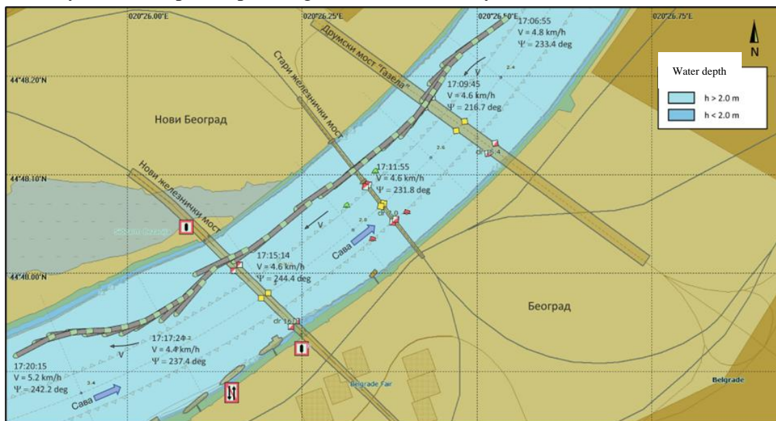
Figure 4.1.1.7. Trajectory of the motor cargo vessel “LEGET III” upon upstream, navigation under the road bridge “Gazela” and the railway bridges
