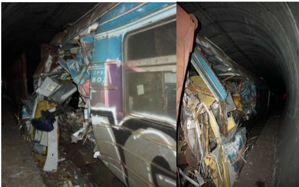
Figure 4.2.1.1: Damage to the front section of motor coach 412-005 of train No. 7112 after the accident
