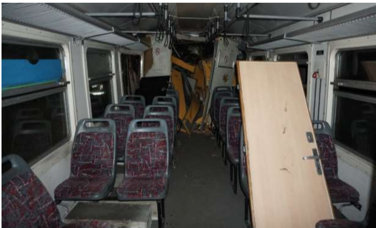
Figure 4.2.1.2: Deformations in the passenger compartment of motor coach 412-005 of train No.7112 after the accident
