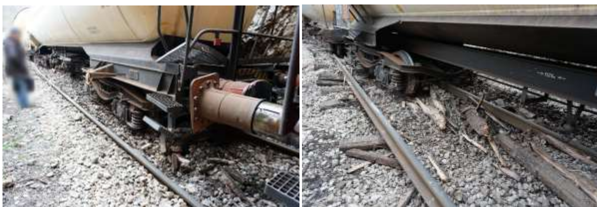
Figure 4.1.1.3: Review of the parts of the derailed wagons
