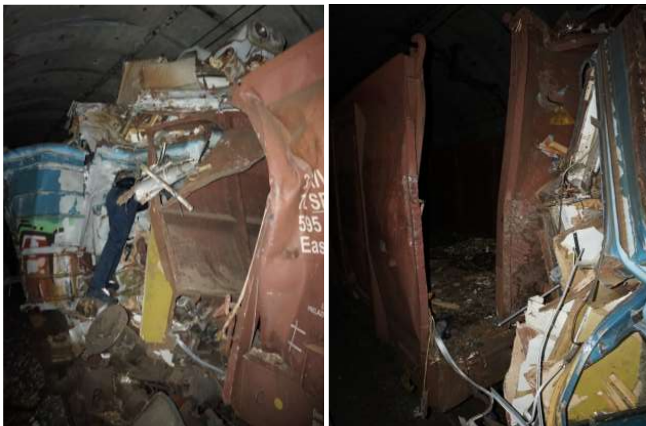
Figure 4.2.1.3: Deformation of wagon No. 31 72 5959 453-7 of train No. 52601 after the accident
