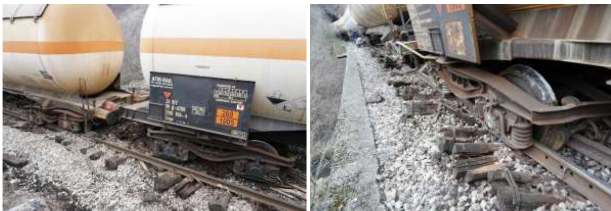
Figure 4.1.1.4: Review of the parts of the derailed wagons
